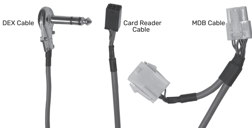
FIGURE 7 G11 TELEMETER CABLES
