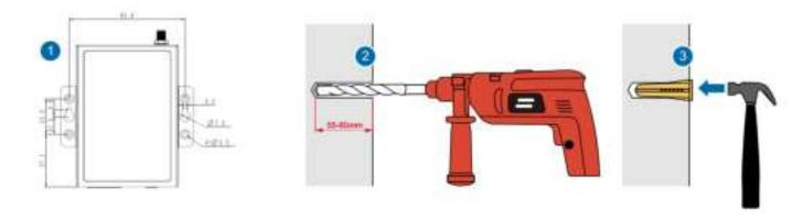
Figure 3: Hole drilling
