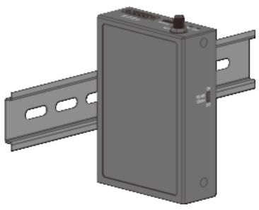
Figure 6: DIN rail mounting
