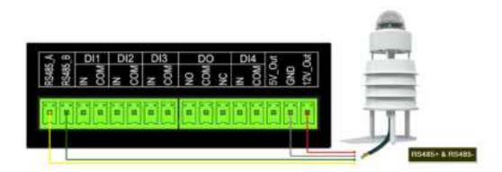
Figure 9: Data interface connection
