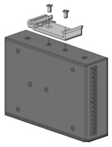
Figure 5: Attaching the clip
