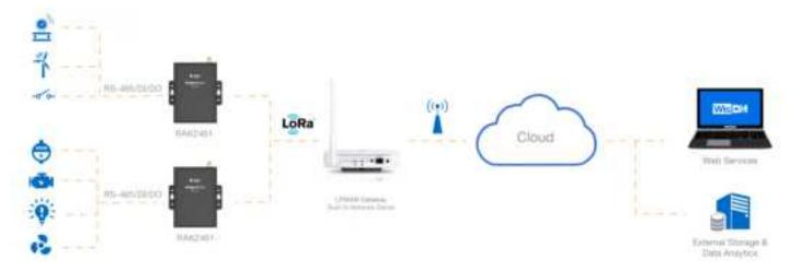
Figure 7: RAK2461 WisNode Bridge IO Lite network structure
