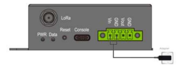
Figure 8: Power interface connection
