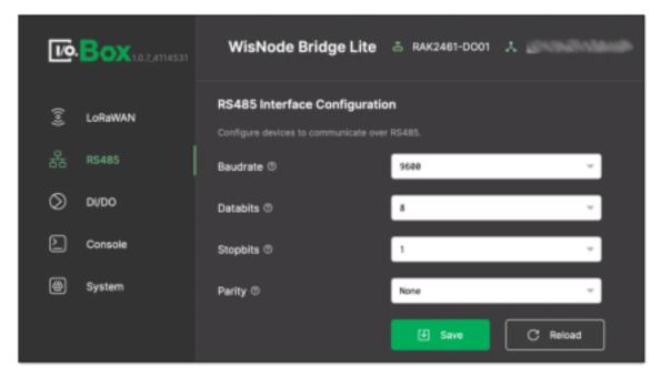
Figure 26: RS485 interface configuration
