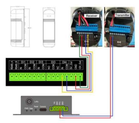
Figure 38: Sensor to Bridge wiring
