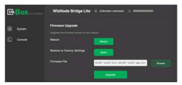
Figure 59: Normal upgrade procedure
