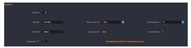
The SpiNode can receive up to 6 universes per port. However, if you patch the maximum number of pixels on one port and do not use 1 as a start address, you will need to receive 7 different universes.
