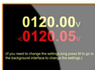
Over-voltage alarm interface
