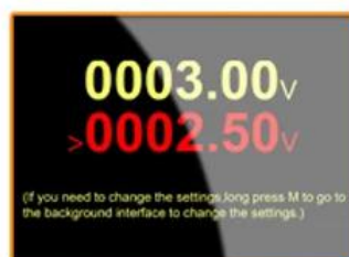
Low-voltage alarm interface
