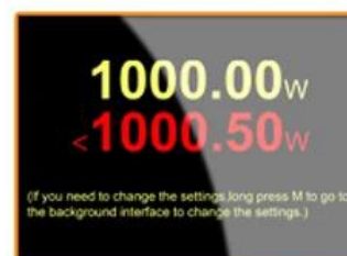
Over-power alarm interface
