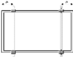
Fig. A1: Clamp position on long frames Mounting rails perpendicular to the longer frame
