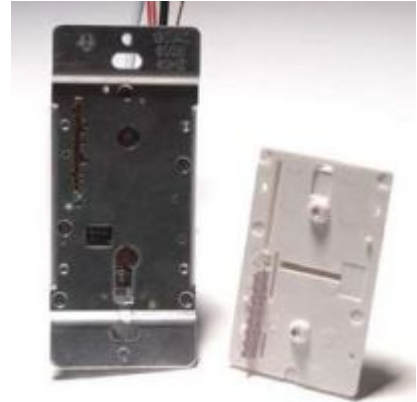
Figure 1: Paddle assembly and SwitchLinc body separated
