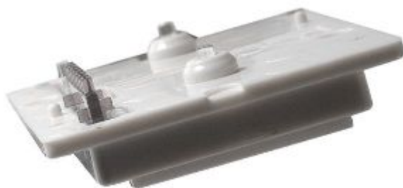
Figure 4: LED light pipes correctly installed
