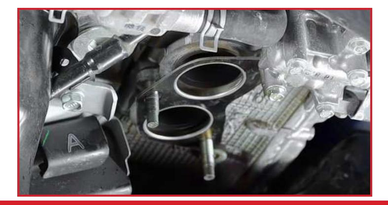
Take your Grimmspeed Header as well as the supplied turbo gasket and lift them up into place under the engine. Loosely install the included replacement nuts onto the studs in the heads, but do not fully tighten them yet. You may need to gently pry the turbo shield to get the header to seat in place on the turbo flange.
