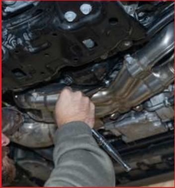
Carefully remove the three turbo studs with an E10 torx socket, taking care not to snap the studs. We highly recommended to use a ratchet instead of power tools to avoid snapping the studs. If you experience resistance, apply penetrating oil and consider heating the area around the studs. We recommend running an M10x1.25 tap through the threads in your turbo to ensure that there is no damage to the threads.
