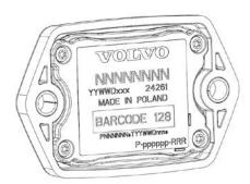
The unit is a rugged wireless unit designed to handle the harsh environments of a construction use case from both vibration and ingress protection perspective. It consists of a durable plastic housing with a removable lid on the back, in order to allow the user to change the battery. It is completely wireless, communicating through Bluetooth Low Power protocol as a peripheral node.
