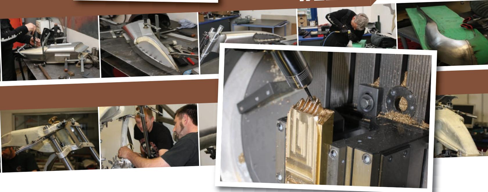
clean without the slightest dent in it. Our forming block was the milled plastic tank. Hours were spent in careful hammering and welding.”
