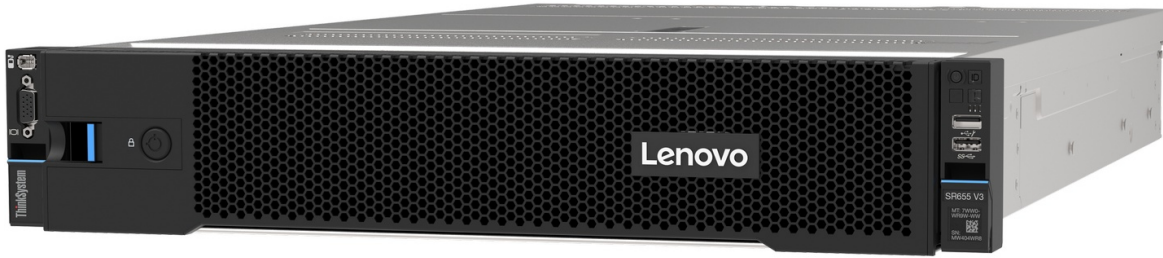
Figure 24. Lockable front security bezel
