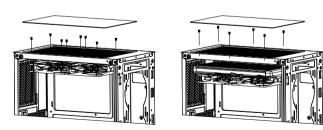
Put fan or water cooling on top panel from inner side and fix screws from outside
