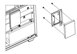
Take off SSD bracket, then fix SSD on bracket and lock bracket to previous place
