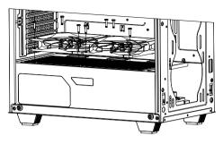
Put fan on upside of psu cover and fix screwss
