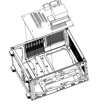
Put M/B to chassis on right position and fix screws
