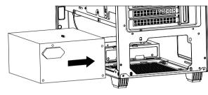
Put psu into chassis from left side
