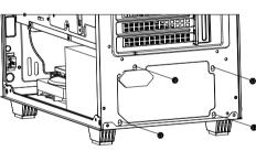
Lock 4pcs psu screws to fix psu
