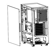
Put side panel on right position and push it, then lock 2pcs screws
