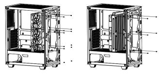
Put fan or water cooling on front plate from inner side and fix screws from outside
