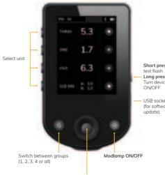
Short press: access to menu Long press: Switch to TTL
