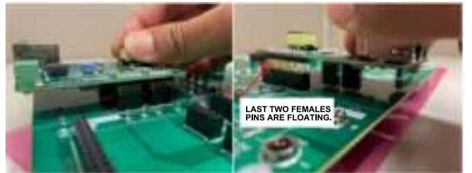
Figure 3. Alignment of an EVAL-10BT1L-MCS-AZ/EVAL-10BT1L-MCS-BZ shield with SPoE PSE Motherboard
