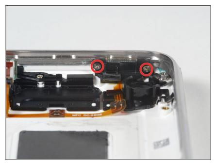
Remove the two Phillips #00 screws securing the on/off switch to the front bezel.
