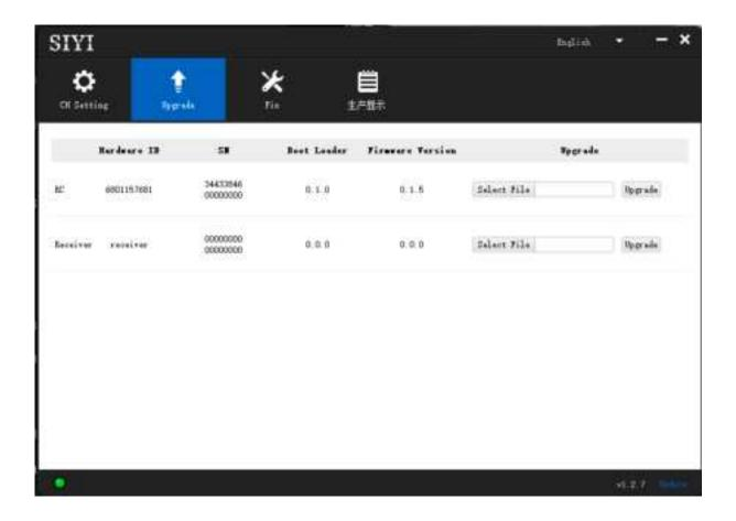
4. If the firmware is not the latest, then click the "Select File" button in the "RC" line to import the latest remote controller firmware. Then click "Upgrade" and wait till it is "100%" finished.
