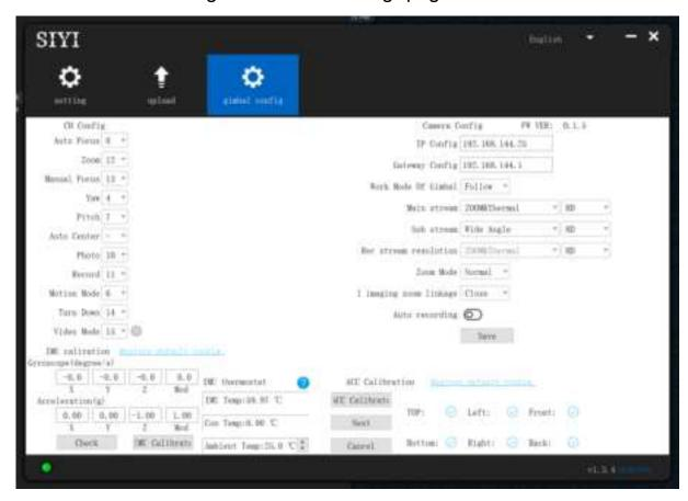
7. Under "Channel Config" page, assign the communication channel 1 to 16 to target gimbal and camera functions according to your requirement.
