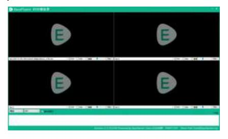
5. Input the complete RTSP addresses of the connected camera or gimbal in Easyplayer to display the video stream.
