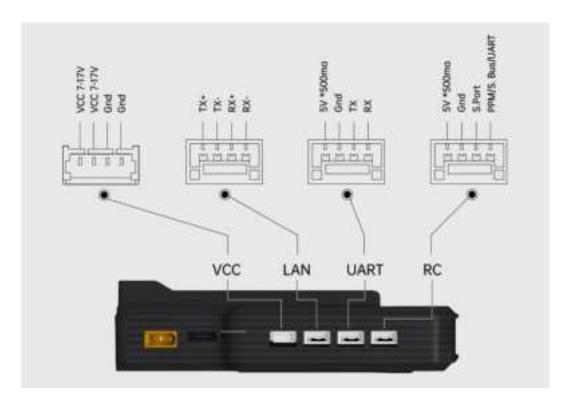
**Ground Unit Interface & Pinouts**
