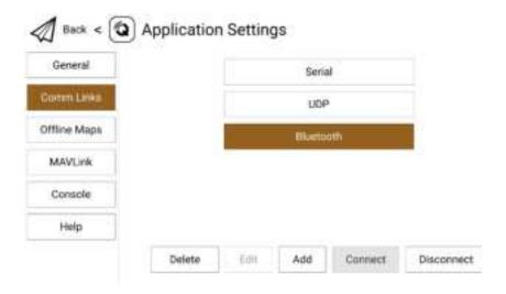
6. Confirm and start to "Connect". The top progress bar in QGC starts to move, which means the remote controller is communicate with QGC automatically. Please wait until the datalink connection is established.
