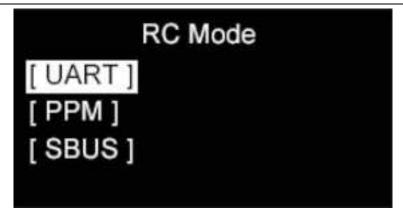
5. Return to the initial page, if there is an "x" icon right after the selected RC input mode, there is no RC signal input through the RC port. If the icon is "←→", there is RC signal input.
