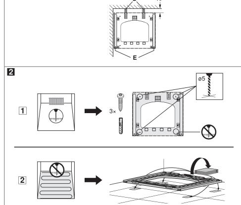
► Fold out spacers **D** in order to keep distance to the back wall.
