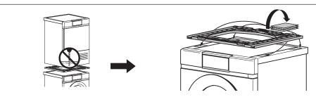
If a tumble dryer has to be installed on top of a washing machine, no holes must be drilled in the washing machine. The installation plate must be adhered to the floor.
