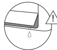
Caution: Do not keep louver at too vertical an angle for long periods of time. This can cause water condensation to drip on your furnishings.
