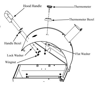
**Step 10:** Insert the Hood Handle through the Handle Bezel and Side Fire Box Lid (from outside) and then through Lock Washers and secure with Wing Nuts as shown below. Install Side Handle on the Side Fire Box with two 1/2" Hex Bolts and two Hex Nuts. Then install the Drawer Latch on Side Fire Box with a 1/2" Hex Bolt and a Hex Nut. **NOTE: Hardware for Handle came attached with Handle.**
