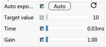
When Auto Exposure is enabled, the target exposure can be set by sliding the "Target Value" bar to the desired value.
