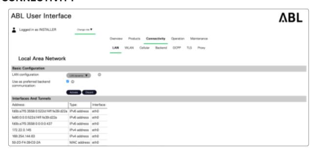
The **Connectivity** tab shows details about the various communication interfaces and protocols within your current installation.
