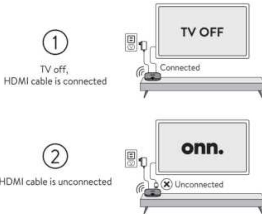
When TV is off or HDMI cable is unconnected, all the sound will be output by Streaming Device itself. (Refer to scenario 1 and scenario 2 above)
