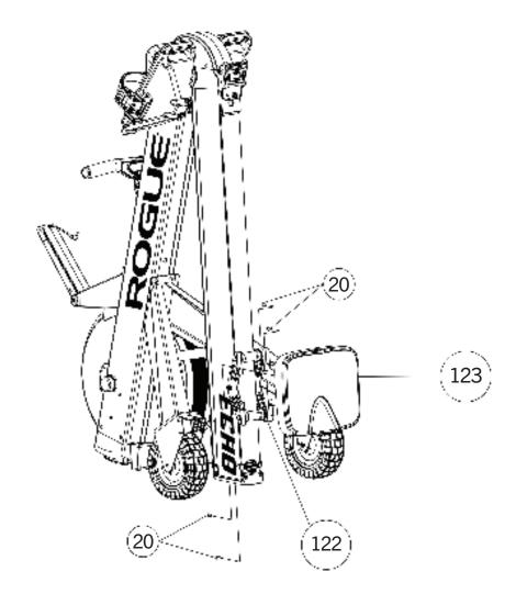
• HOLD TIRE WITH YOUR FOOT WHEN UNFOLDING THE UNIT BY SEPARATING THE REAR MAIN FRAME ASSEMBLY FROM THE FRONT FOOT TUBE ASSEMBLY
