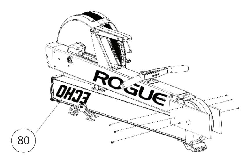
• ASSEMBLE THE END CAP (33) ONTO THE FRAME (80)
