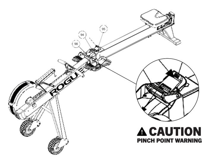
• LIFT THE REAR LATCH (95) UP BY HAND, AND THE ENTIRE BUCKLE WILL BE RELEASED, ALLOWING THE FRONT AND REAR FRAMES TO FOLD UP
