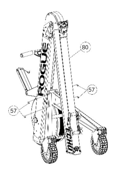
• FIX THE LEFT (L) AND RIGHT (R) FOOT PEDAL ASSEMBLIES TO THE FRAME (80) USING A 1/4-20 FULL THREAD SCREW (83) (PAN HEAD SCREW)
