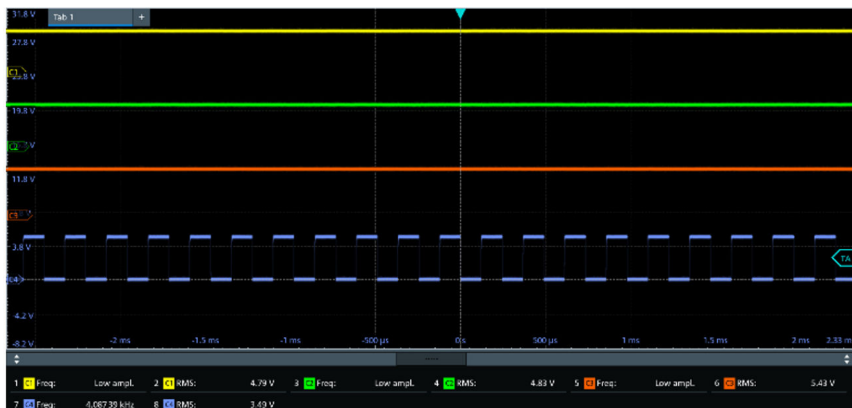
Figure 26. Overvoltage status for LDO2
