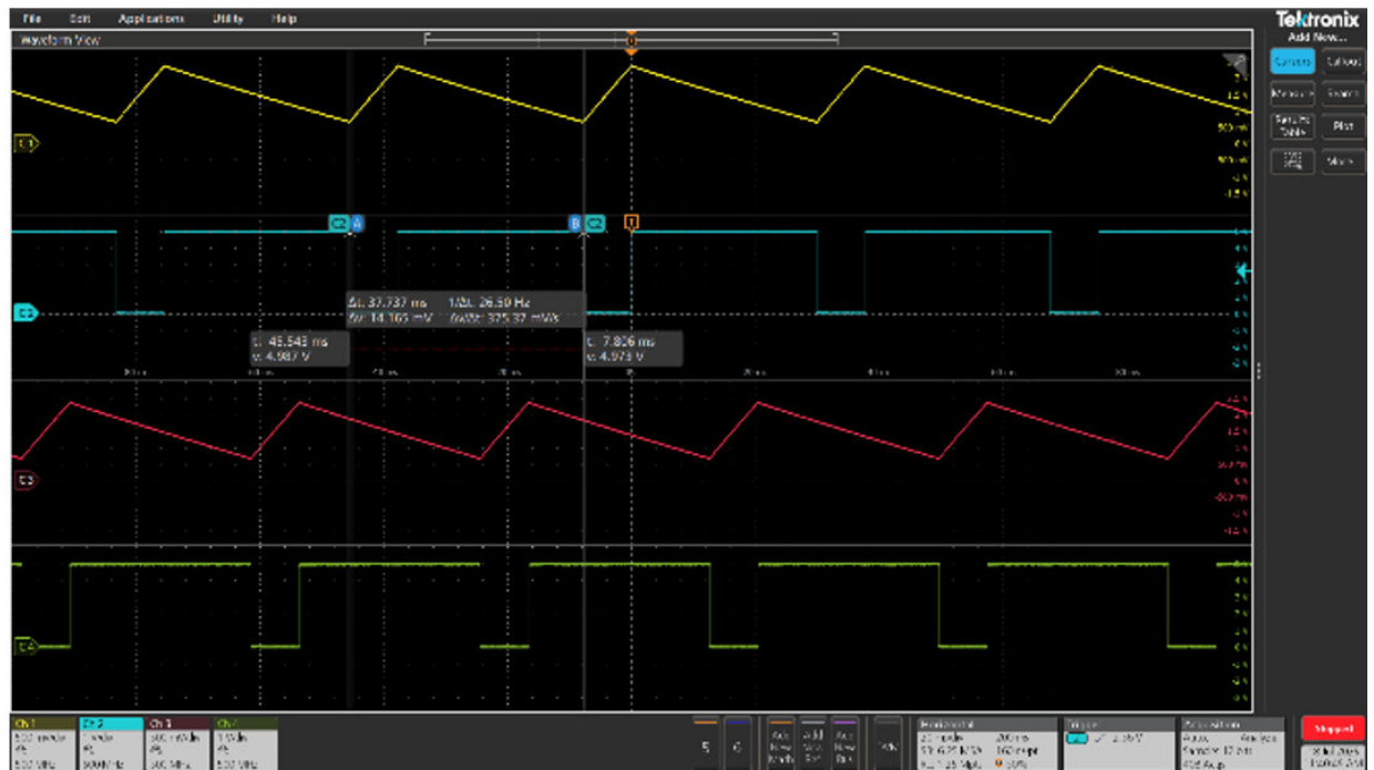
Figure 22. RS_LDO1 without Wi_LDO1 for VO1 output (VO1= 5V F=26.50Hz)
