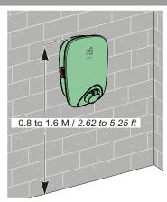
■ Check the installation area before marking it on the wall. It is recommended to situate the top of the charging station between 0.8 to 1.6 m / 2.62 to 5.25 ft above the ground.
