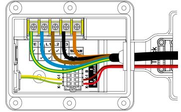
Note: Please ensure all 3 phases are connected correctly Power supply cable from the bottom side.
