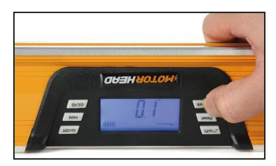
4. Flip the level over, press "calibration" button till it beeps, now level is calibrated ready.
