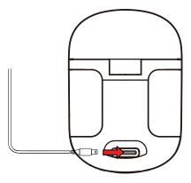
Insert the other end of the USB cable into a suitable USB charging adapter.
