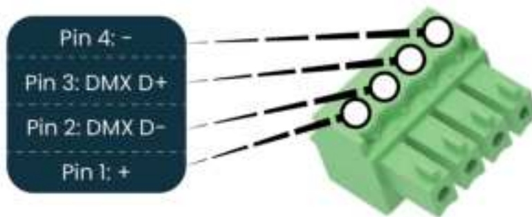
Figure 12: Pixel Output Pinout for Differential DMX512 Pixels
