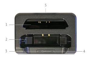
The Desktop Charger IS-DC540.1 allows you to charge a device and its spare batteries simultaneously.
