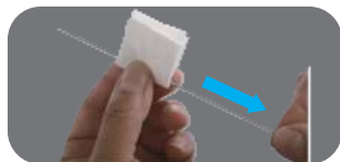
4. Fold a soft cloth damp with cleaner over the needle, wipe the residual paint off.
