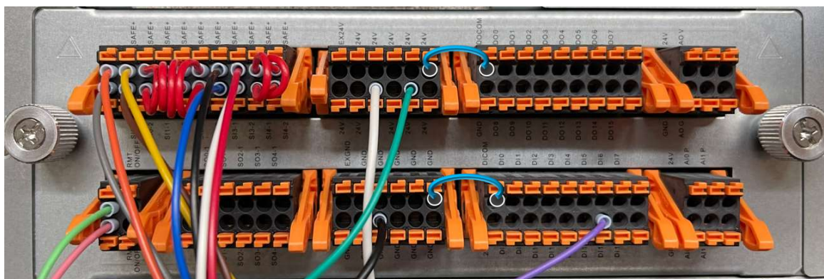
Connecting junction wires (PNP type) to OMRON/ TM control box
