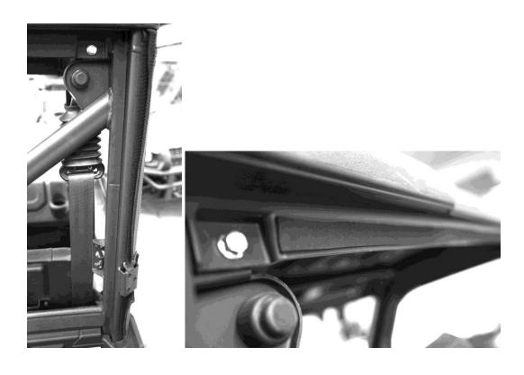
9. Now that the padding and bottom brackets are in place it's time to place the Rear Window in place on the vehicle. The brackets are designed to hold the window in place along the bottom of the frame in behind the seats as shown in the photo below.
