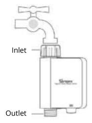
First, wrap the thread seal tape around the thread of the faucet, then screw the nut of the water inlet of the equipment onto the faucet. After testing that there is no leakage, finally connect the hose to the water outlet of the equipment (if the water outlet leaks, please wrap thread seal tape around the thread of the water outlet).
