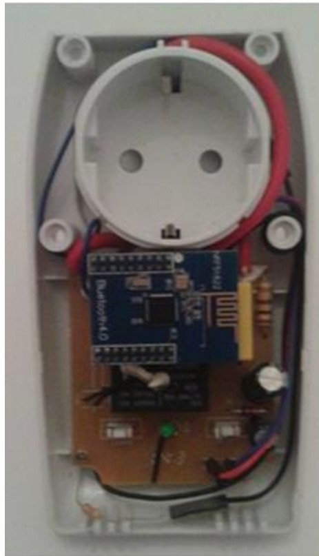
Figure 4.8 – Adapted Smart Plug with Core51822.
