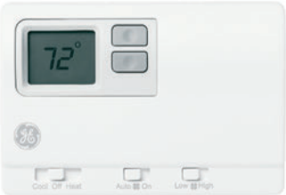
RAK149F2 HEAT PUMP DIGITAL TWO FAN SPEED THERMOSTAT • Two fan speeds • 24V AC digital remote wall thermostat • Requires 6-wire (resistance heat) or 7-wire (heat pump) hookup • Works with single-stage cooling and single-stage or two-stage heating systems
