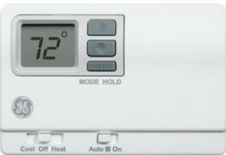
RAK149P2 HEAT PUMP DIGITAL PROGRAMMABLE REMOTE THERMOSTAT • 24V AC digital remote wall thermostat • Programmable for 7-day or 5+2-day programs • Requires 5-wire (resistance heat) or 6-wire (heat pump) hookup • Works with single-stage cooling and single-stage or two-stage heating systems • One fan speed
