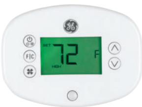
RAK180W1 ENERGY MANAGEMENT OCCUPANCY SENSING WIRED/ WIRELESS THERMOSTAT • 2-wire power connection available (all other signals wireless) • Thermostat (shown) & control card (mounts on top of unit) included • Control card works off 24V AC signal from unit • Works with single-stage cooling and single-stage or two-stage heating systems with proper setup. Default is two-stage heating and B-type heat pump • Extra 24V output may be programmed to control other room systems such as lighting, vents, etc.
