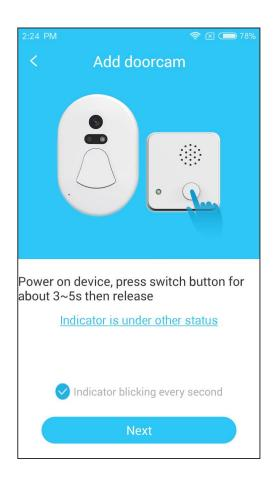
Note: If the indicator does not flash at once per second, please reset the indoor unit. 【Reset method: Long press the function key for 3 ~5s release】
