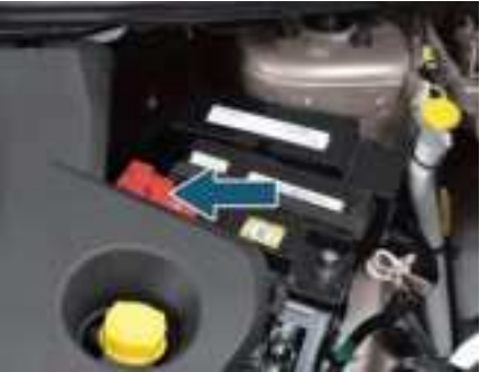
Motor Compartment Fuse Box
