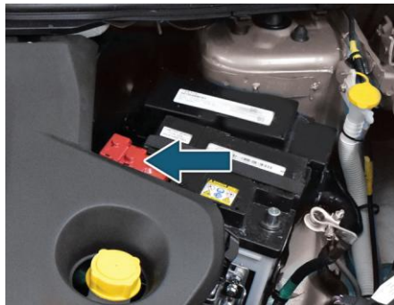
Motor Compartment Fuse Box
