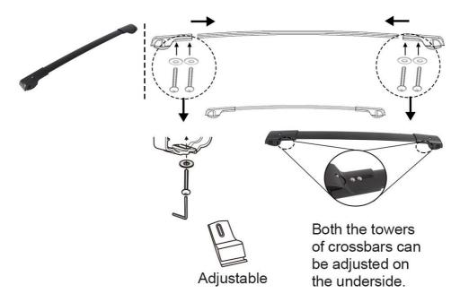
1. First, install and fix the left and right adaptor on the left and right sides of the front and rear aluminum tubes, respectively, and fix them with M6 screws+M6 spacer; then install them to the roof rack as shown in the picture.
