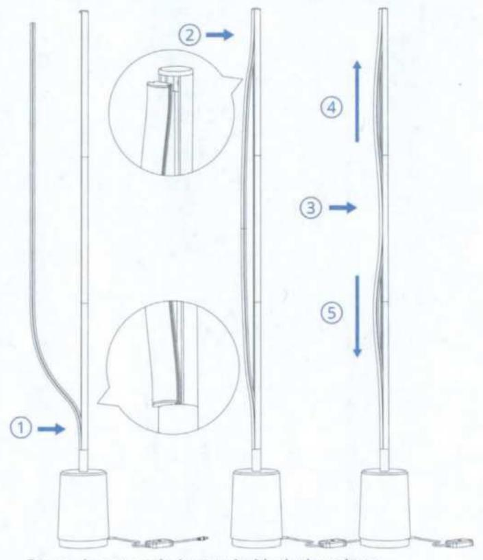
Ensure the exposed wires are inside the lamp base. Attach the silicone strip light by following the image above. Finally press the strip light from the middle outwards to the two ends.
