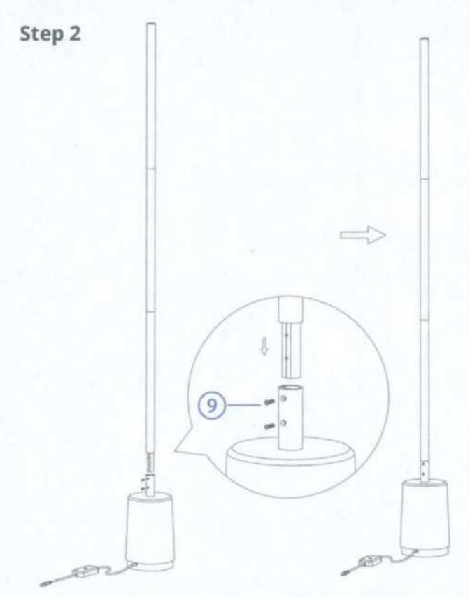
Connecting the lamp pole and lamp base: Insert the connected lamp pole into the lamp base. Use the long screws to secure the final connecting part via the two holes on the base.
