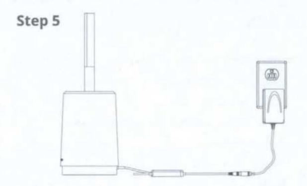
Connect the adapter to the cable of the lamp base and plug the adapter into a socket. Then you can start using the product.
