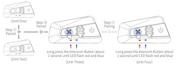
Click the Intercom Button on either unit to search and pair the other unit, the LED light flash blue quickly. Once pairing is completed, the LED will blink blue slowly on these four units.
