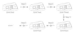
**Note:** Each B4FM device can only be paired with two other B4FM devices at the same time, that means, we pair the unit one after another in series to realize multiple group connections. For example, if unit three is paired with unit two and unit four, and it will not be able to pair with other devices.
