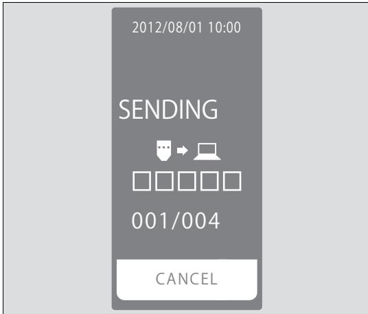
Display shows the number of data transferred and the number of data in memory to be transferred. It also shows the progress of the transfer of all data in memory.
