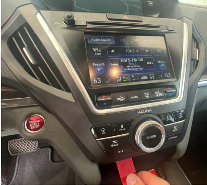
1. Using a plastic tool, pry underneath the navigation screen control panel.
