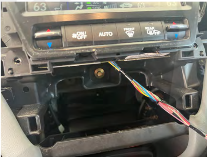
4. Remove harness connected to controller panel.
