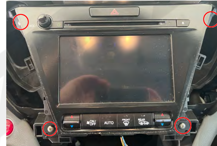
3. Remove (4x) screws securing radio (lower screen) from sub-dash.
