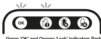
Green 'OK' and Orange 'Leak' indicators flash
