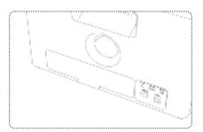
There is a small latch on the bottom of the unit that keeps the battery in place. When installing the battery, insert the tabs on the left first, and push the battery in until the latch clicks. To remove the battery, pull the catch on the latch outward.
