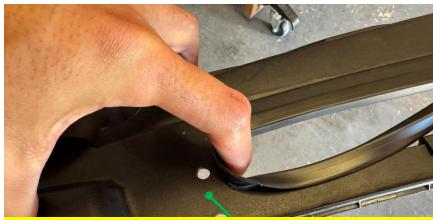
Push into the short edges of the cut plastic to leave no gap
