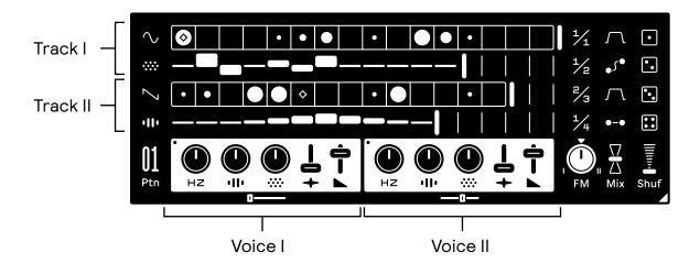
The sequencer has both a trigger (top) and modulation (bottom) track with individual length and tempo division. The trigger track sends velocity and note-on to the voice while the modulation affects the main five voice parameters.
