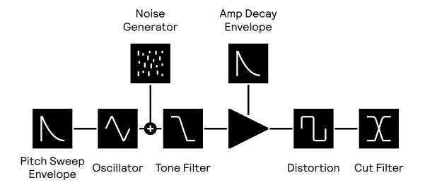
The synth voices in Dyad use a type of virtual analog synthesis with thru-zero linear FM and variable waveshapes. It's configured as a simple one oscillator voice inspired by vintage analog percussion synths, with an emphasis on utilizing the sequencer modulation and bi-directional FM for sound design.
