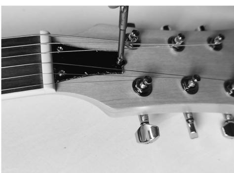
Screw the truss rod cover onto the headstock.
