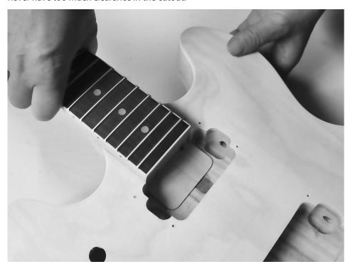
Turn the guitar over. First put on the rubber plate, then position the neck plate over the four screw holes on the back of the body. Then screw the four long wood screws provided through the holes in the neck plate, body and neck until everything fits tightly.
