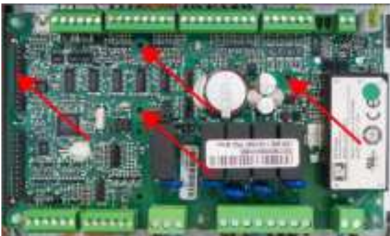
3. The expansion PCB must be connected to connector CN9, and the caps must be mounted in the holes provided for this on the CTS602 circuit board.
