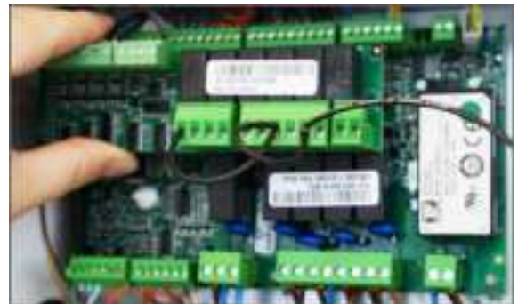
4. Mount the expansion PCB on the CTS602 circuit board.
