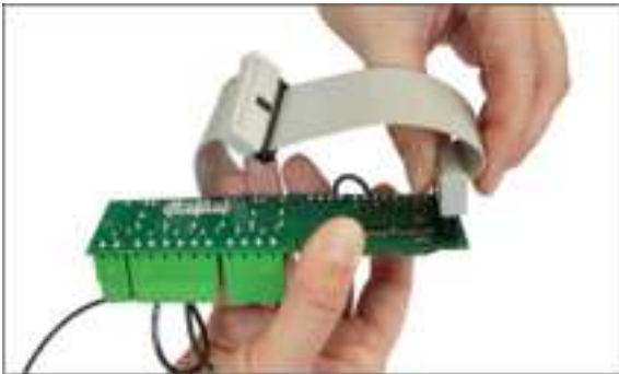
1. Remove the shown bus cable on the expansion PCB.
