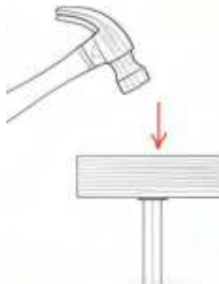
**Tip:** To avoid damaging the sleeve, place a piece of wood on top of the sleeve as illustrated, and gently hammer the sleeve down into the hole until it sinks into the ground.
