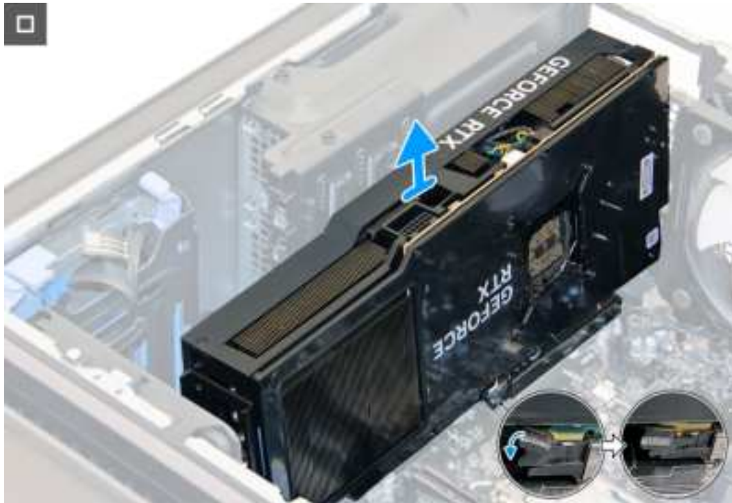
Figure 31. Removing the single-graphics card
