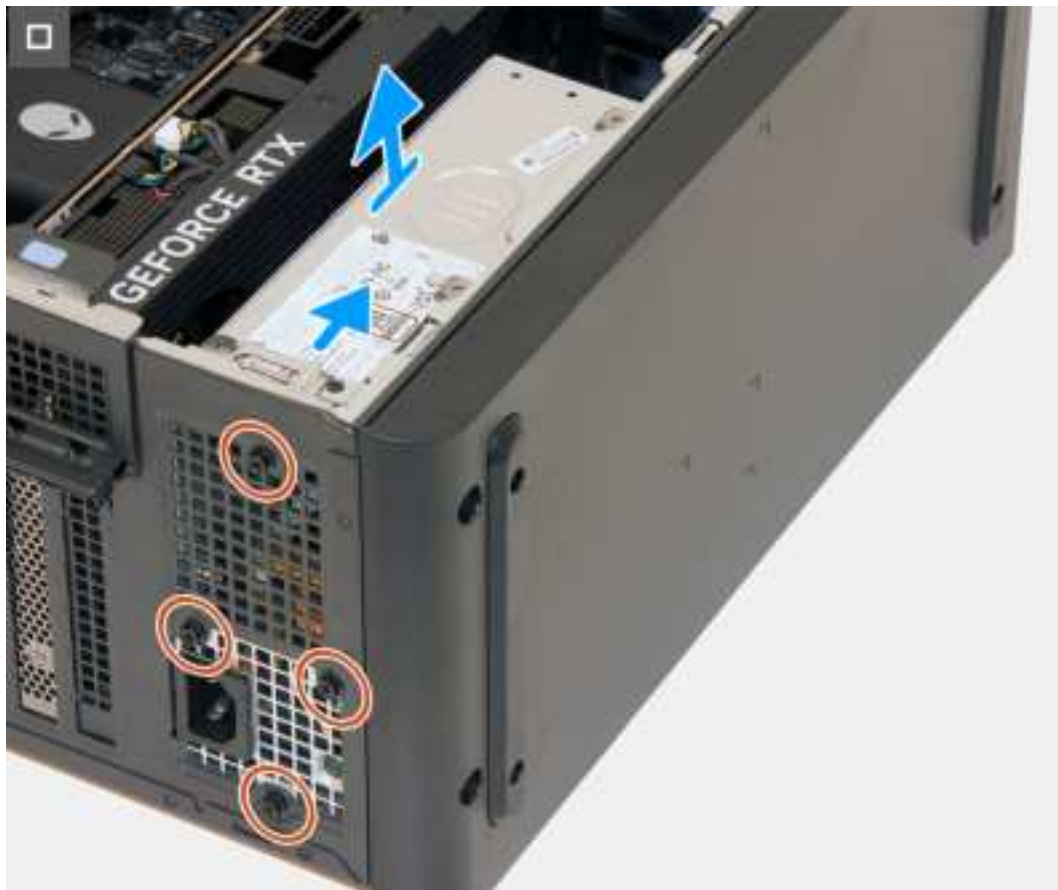
Figure 46. Removing the power-supply unit
