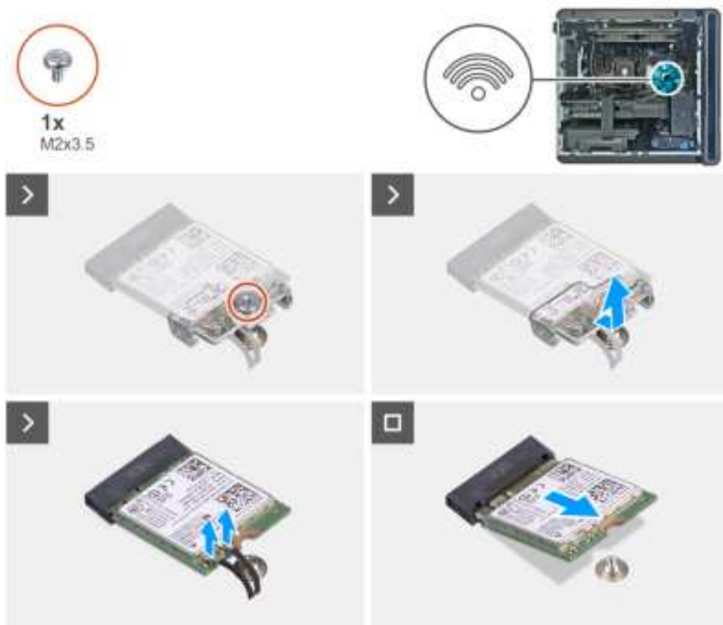
Figure 39. Removing the wireless card
