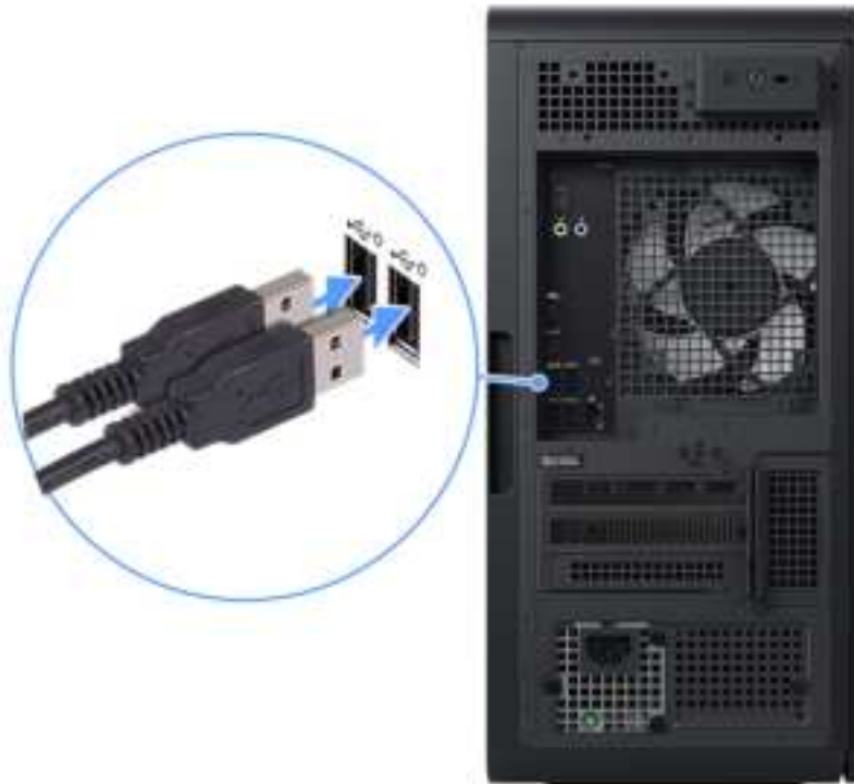
Figure 7. Connecting the wired keyboard and mouse
