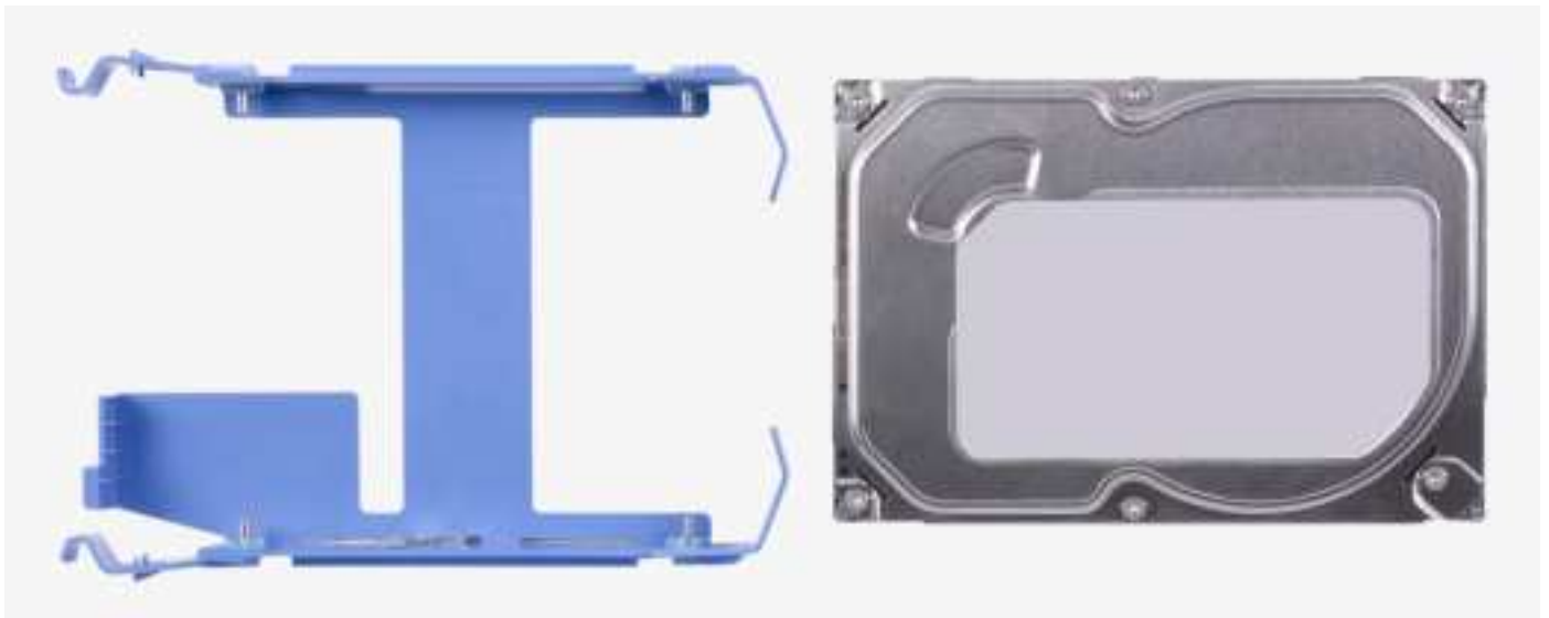
Figure 24. Hard drive and hard-drive carrier
