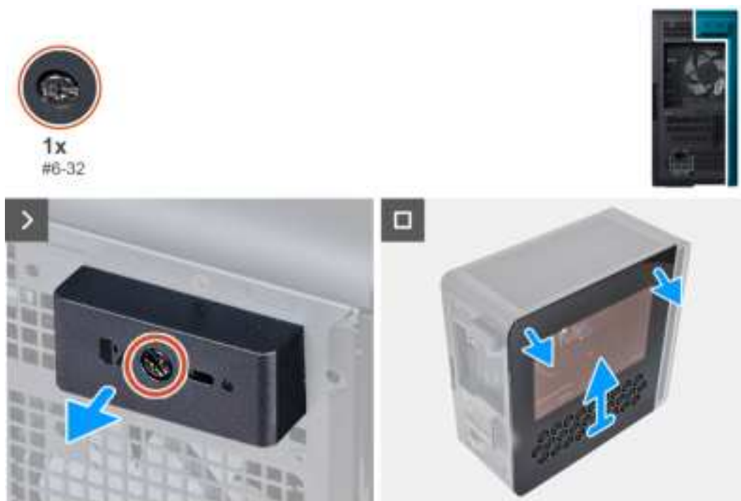
Figure 14. Removing the left-side cover
