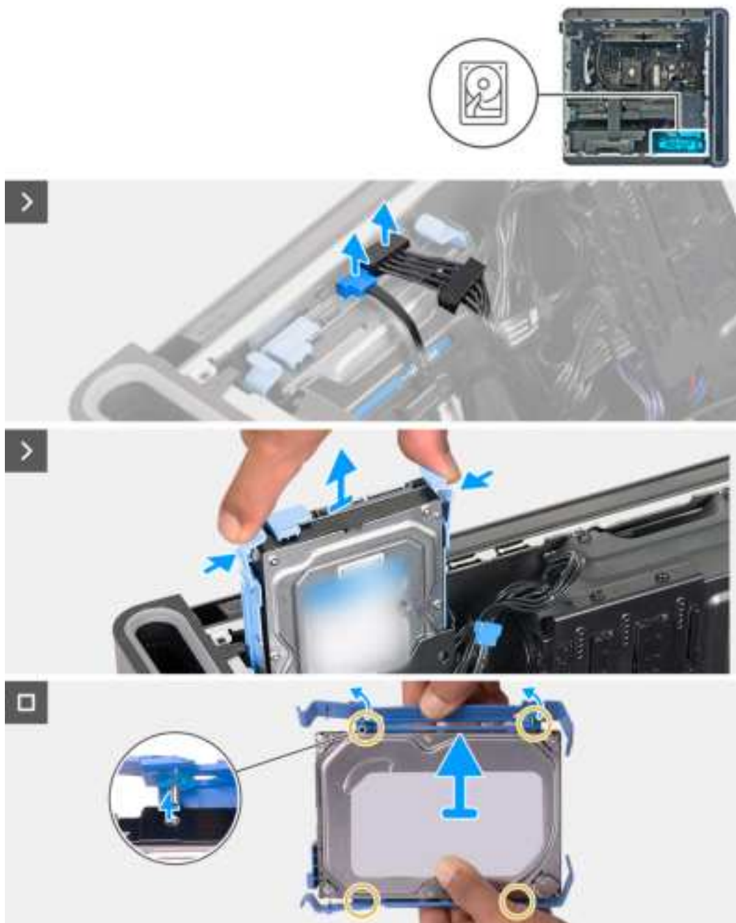
Figure 22. Removing the 3.5-inch hard drive
