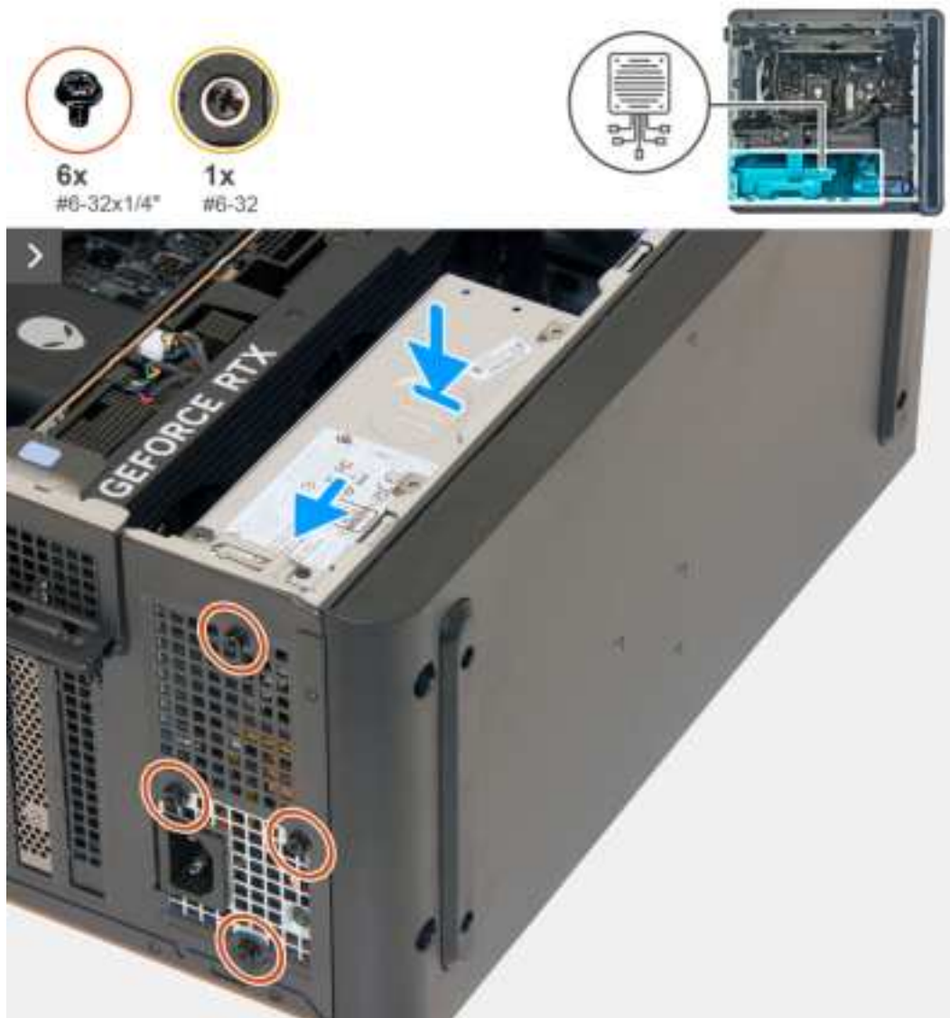
Figure 47. Installing the power-supply unit
