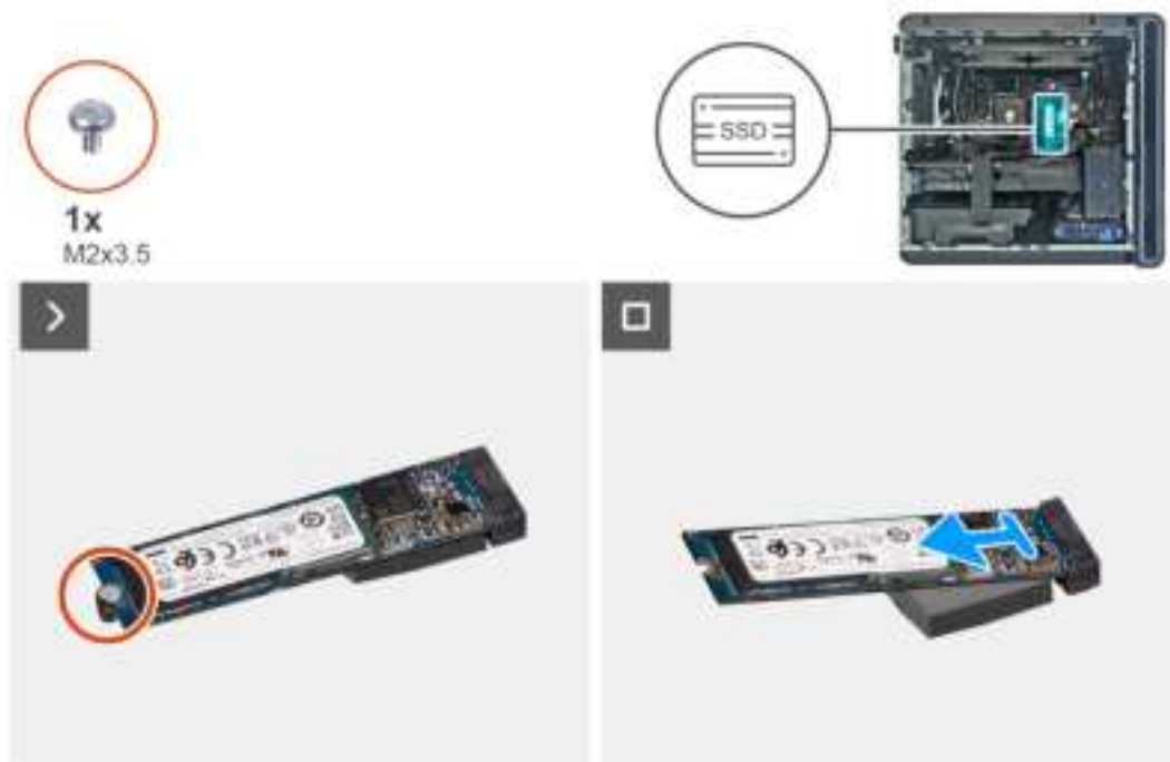
Figure 36. Removing the M.2 2280 solid state drive
