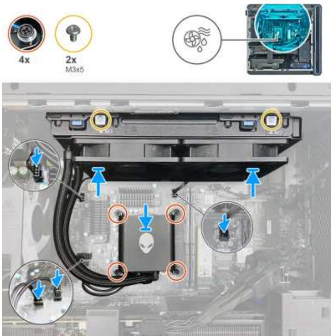
Figure 52. Installing the processor liquid-cooling assembly
