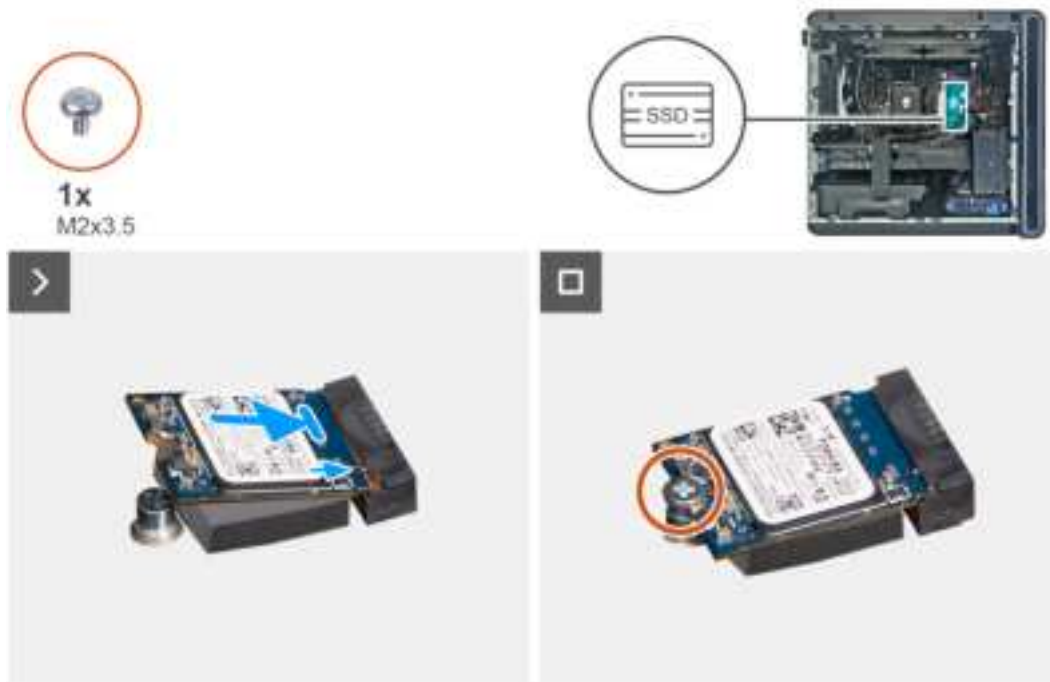
Figure 35. Installing the M.2 2230 solid state drive
