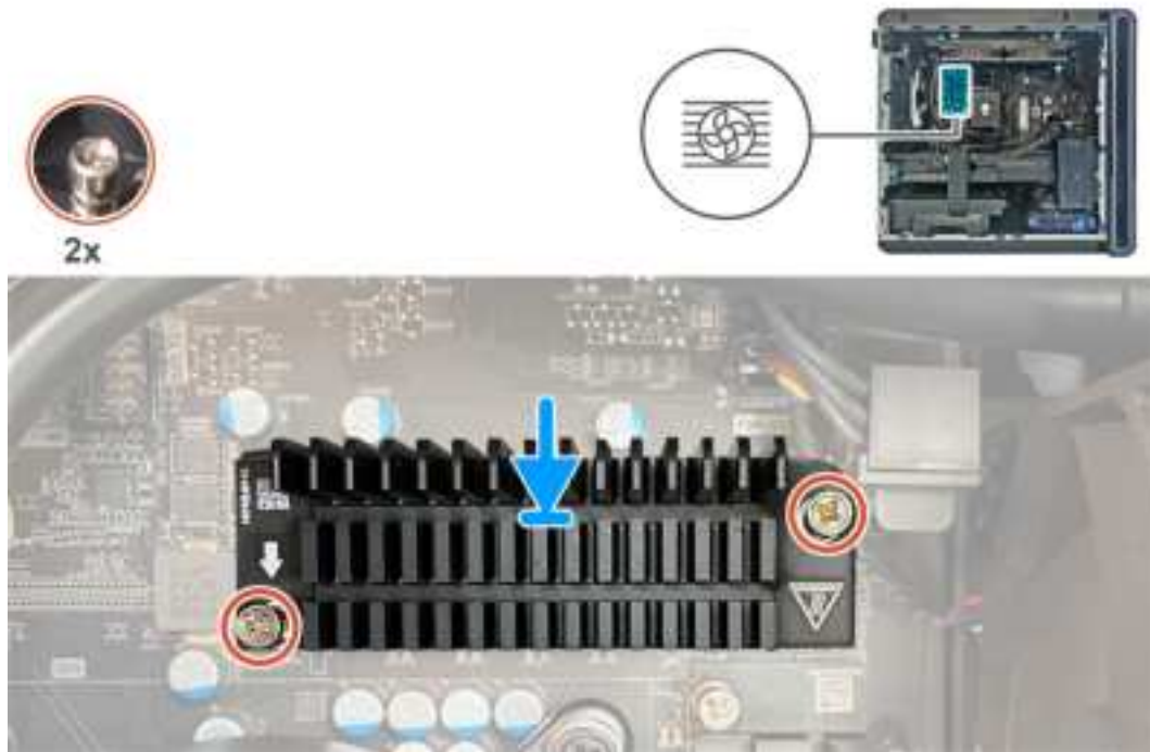
Figure 61. Installing the VR heat sink
