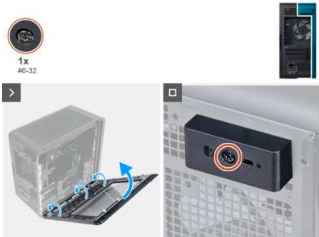
Figure 15. Installing the left-side cover
