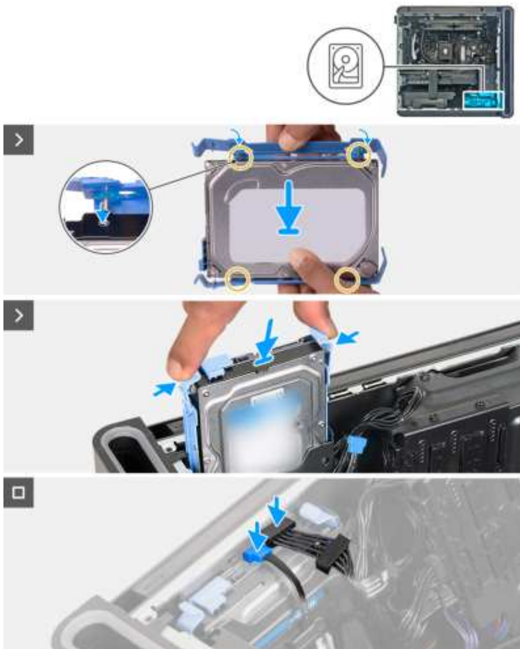
Figure 25. Installing the 3.5-inch hard drive
