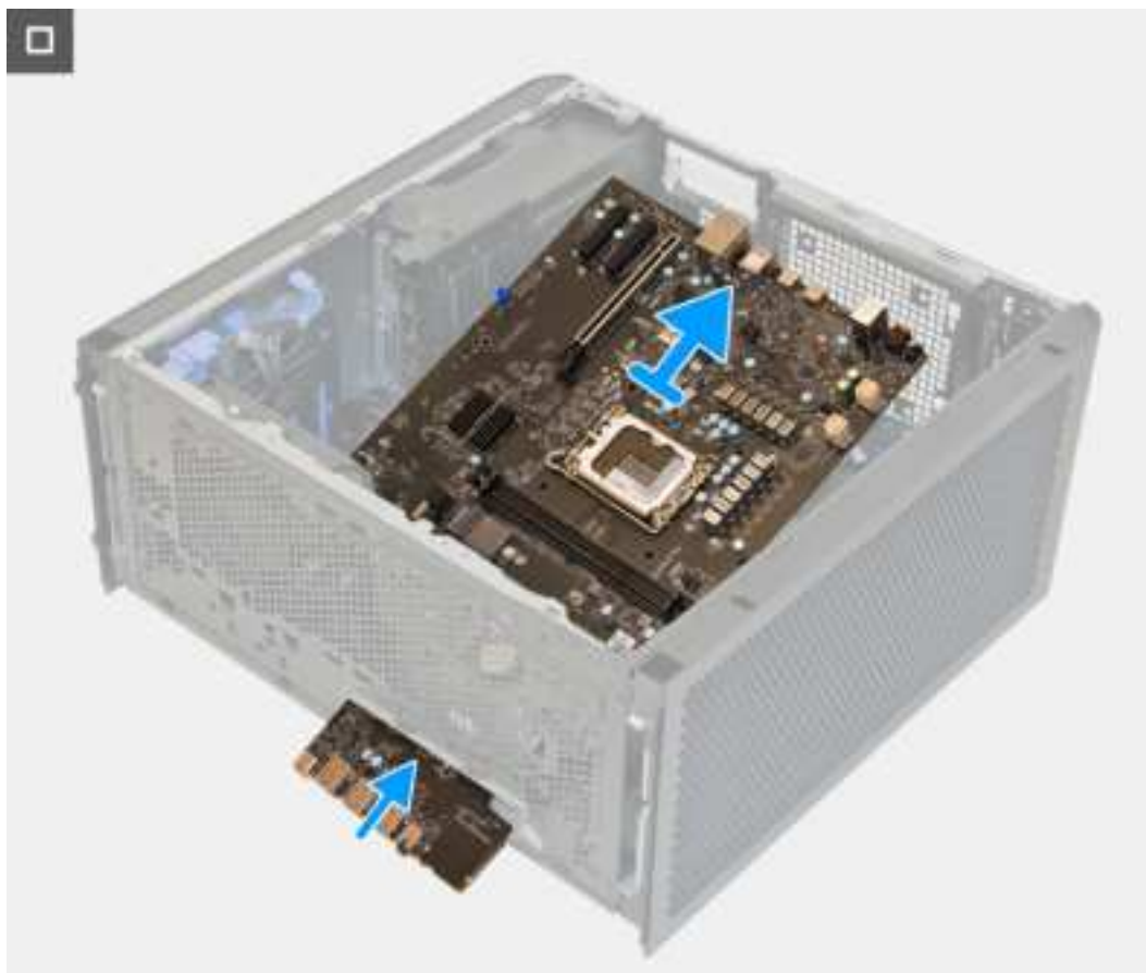
Figure 65. Removing the system board
