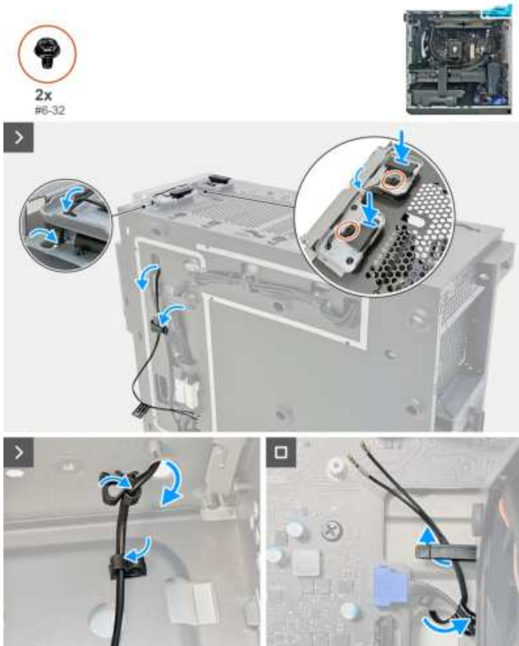
Figure 58. Installing the antenna
