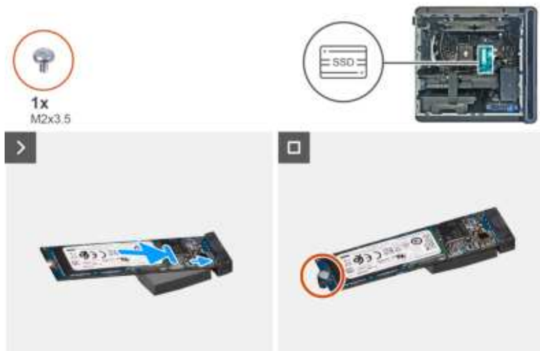
Figure 38. Installing the M.2 2280 solid state drive
