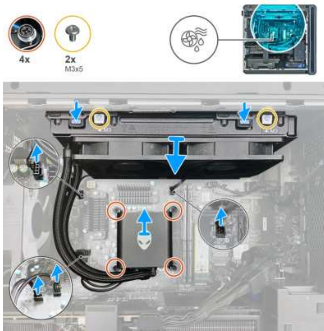
Figure 51. Removing the processor liquid-cooling assembly
