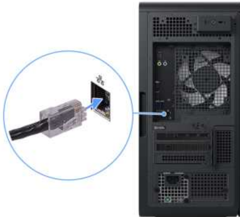
Figure 8. Connecting the Ethernet cable
