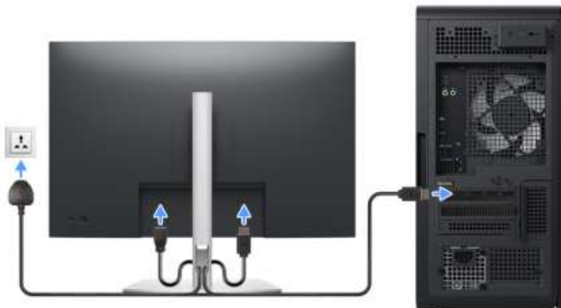
Figure 9. Connecting the display
