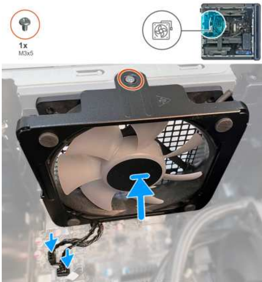
Figure 44. Installing the rear-chassis fan
