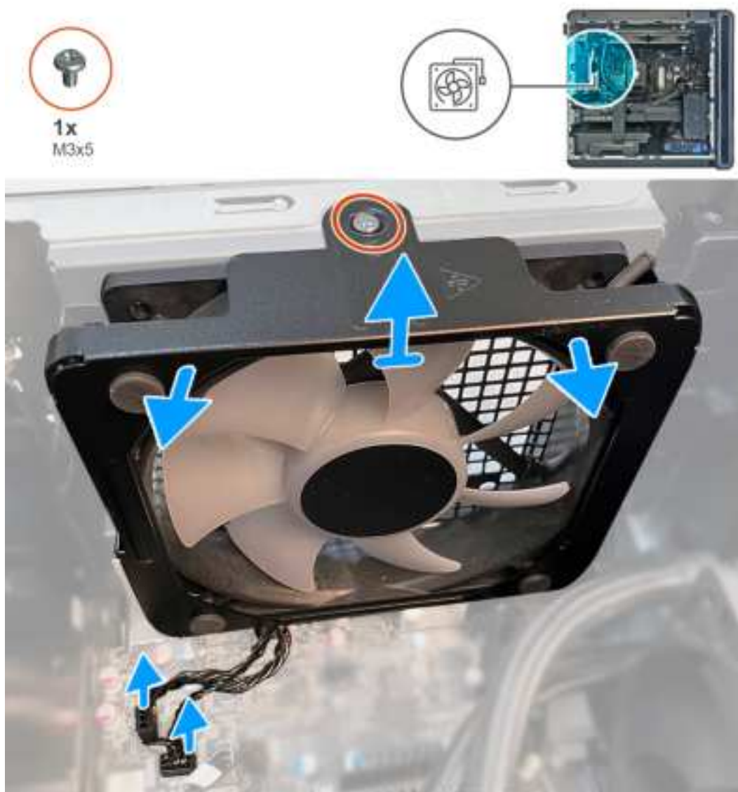
Figure 43. Removing the rear-chassis fan
