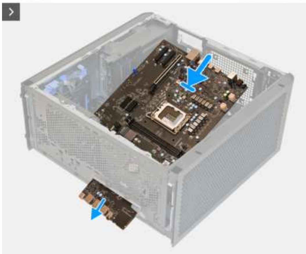
Figure 67. Installing the system board
