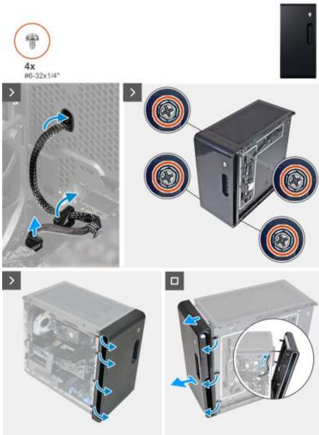
Figure 18. Removing the front bezel
