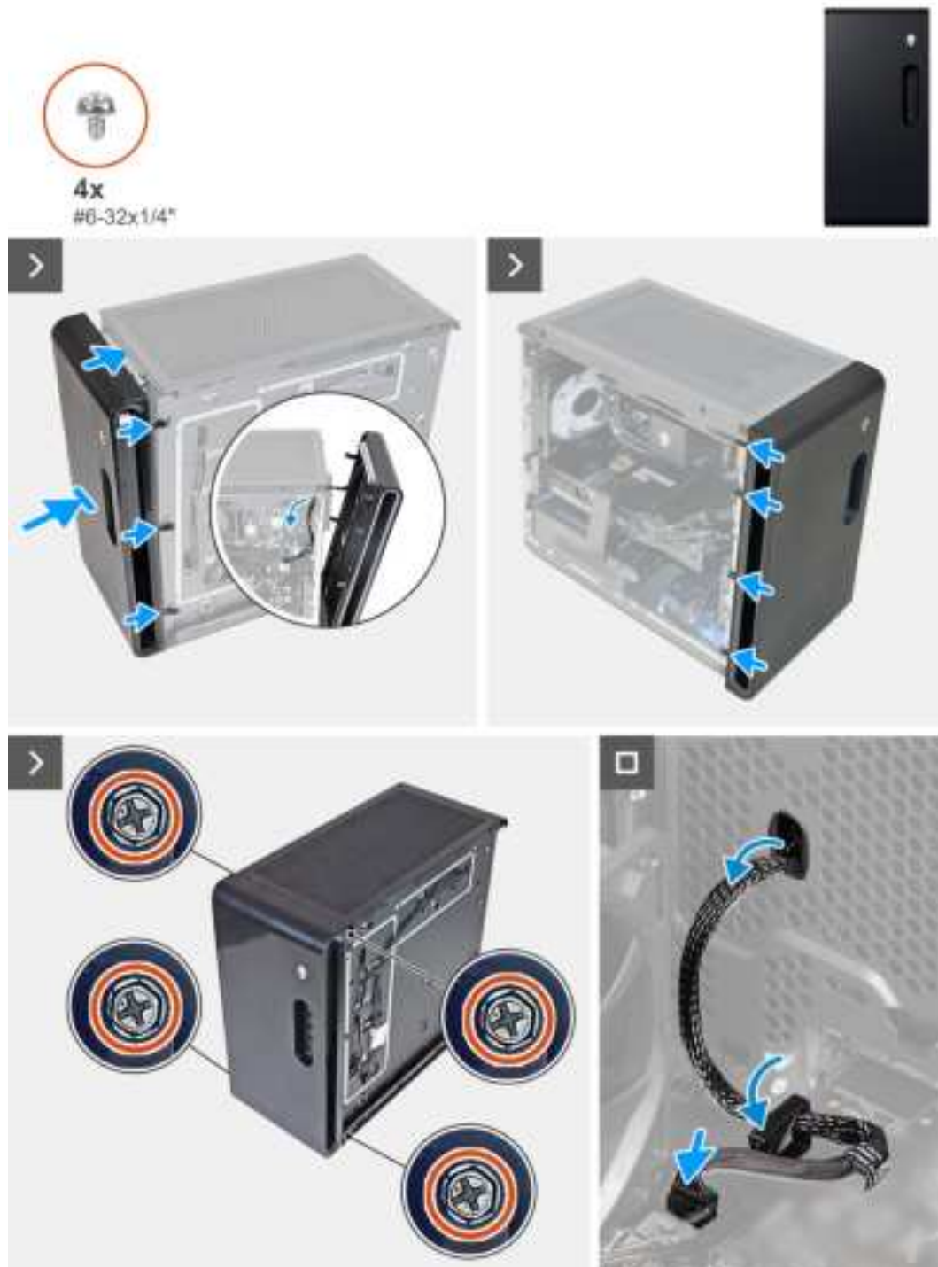
Figure 19. Installing the front bezel
