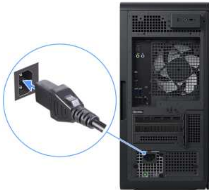
Figure 10. Connecting the power cable
