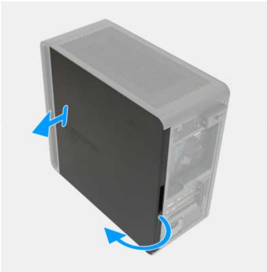
Figure 16. Removing the right-side cover
