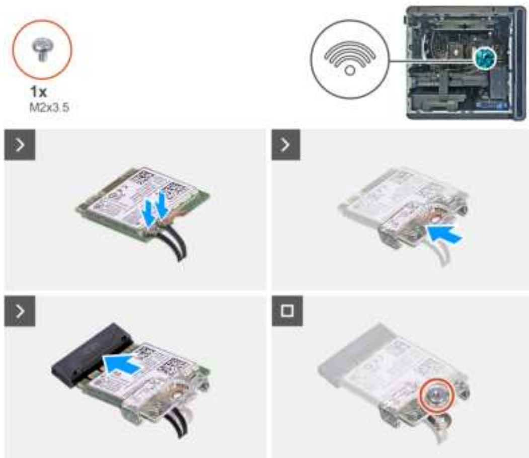
Figure 40. Installing the wireless card
