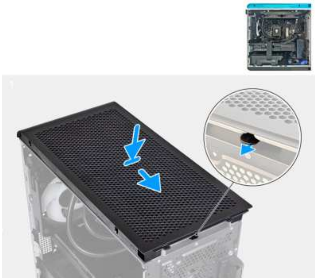
Figure 21. Installing the top cover
